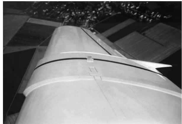
Figure 5. LDV probe during in-flight tests.
