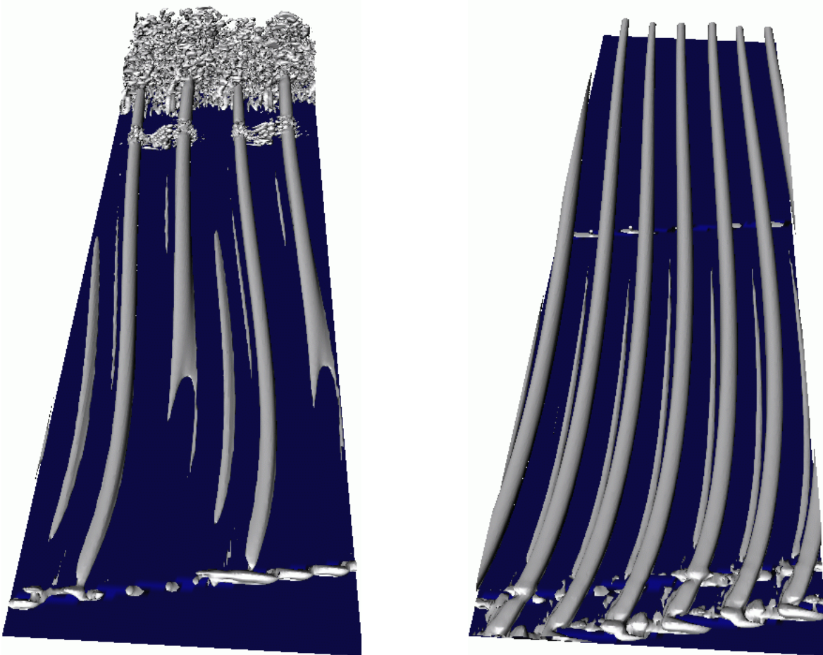
Figure 2. Snapshots of vortical structures. Left: like fig. 1, but in an extended domain. Right: with upstream flow deformation (UFD), i.e. appropriately enforced narrow-spaced vortices. Transition is shifted far downstream because the background pulses do not grow anymore.
