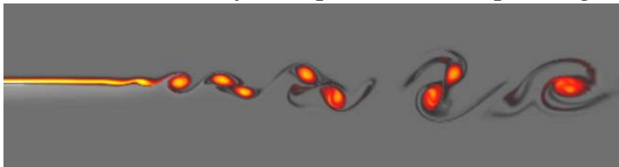
2-d shear wake after a plate: vortex pairing
