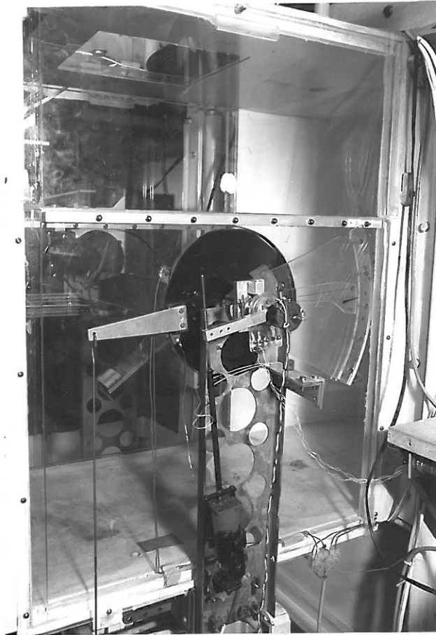
Fig.5 : Test section of the Modelwindtunnel Flow direction is from right to left. The dark painted model is mounted horizontal.
