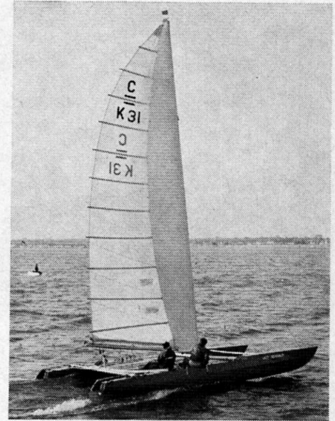
Fig. 1 Racing catamaran «Lady Helmsman» with airfoil mast and sailcloth extension
