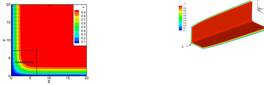
Fig. 1 Numerical solution of the self-similar corner equations. The shaded area indicates the region where a hypothetical laboratory uncertainty might appear.
