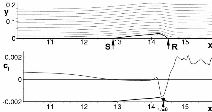
**Figure 2:** Illustration of time-averaged streamlines and wall-friction coefficient.
