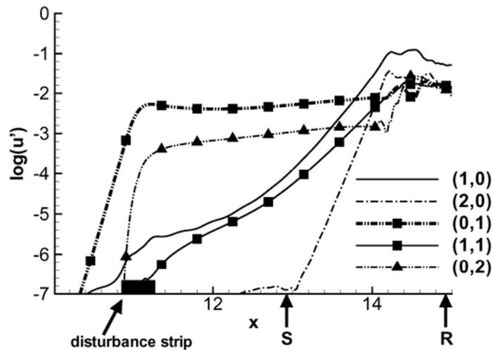
**Figure 6:** Disturbance amplification of selected modes for the case with steady 3D forcing
