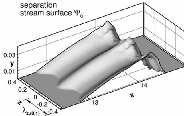
**Figure 7:** Time averaged separation stream surface for the case with steady 3D forcing
