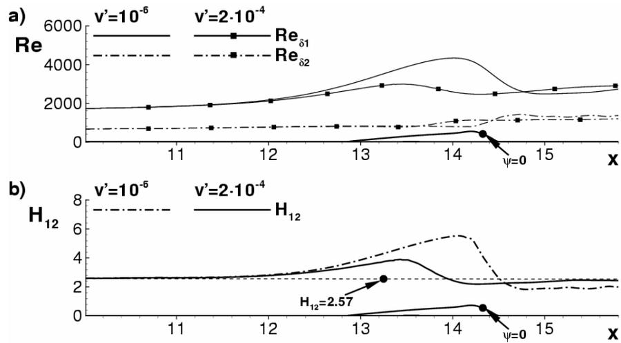
**Figure 5:** Comparison of Reynolds numbers based on displacement thickness ( $\delta_1$ ) and momentum thickness ( $\delta_2$ ) as well as the shape factor  $H_{12} = \delta_1/\delta_2$  for the case with smallest and with largest forcing amplitude.
