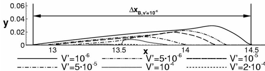
**Figure 4:** Separation streamlines for different wall-forcing amplitudes
