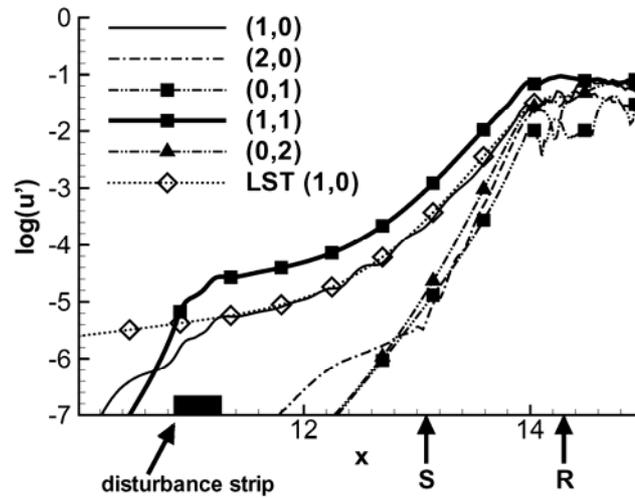
**Figure 8:** Disturbance amplification of selected modes for the case with unsteady 3D forcing
