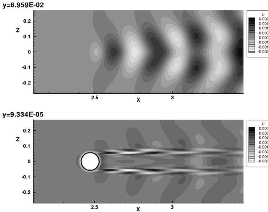
Figure 2. Disturbance field created by interaction of a periodic free-stream perturbation with the roughness element; top: far away from the wall ( $y = 8.14 \delta^*$ ), bottom: close to the wall ( $y = 0.011 \delta^*$ ).
