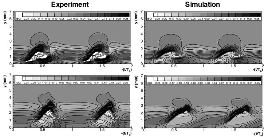
**Fig. 2.** Comparison of the spanwise vorticity component of experiment (left column,  $\omega'_z \approx \frac{\partial u'}{\partial y}$ ) and simulation (right column,  $\omega'_z = \frac{\partial u'}{\partial y} - \frac{\partial v'}{\partial x}$ ) at 1-spike stage. Top row  $\Delta z \approx 2 \text{ mm}$  off-peak, bottom row at peak position  $z = 0 \text{ mm}$
