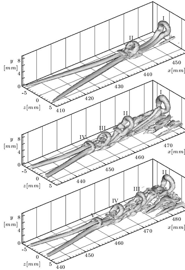
**Fig. 1.** Iso-surfaces  $\lambda_2 = -200$  for three time instants,  $t/T_0 = 0.335$ ,  $0.605$ , and  $0.845$ , from top to bottom, respectively
