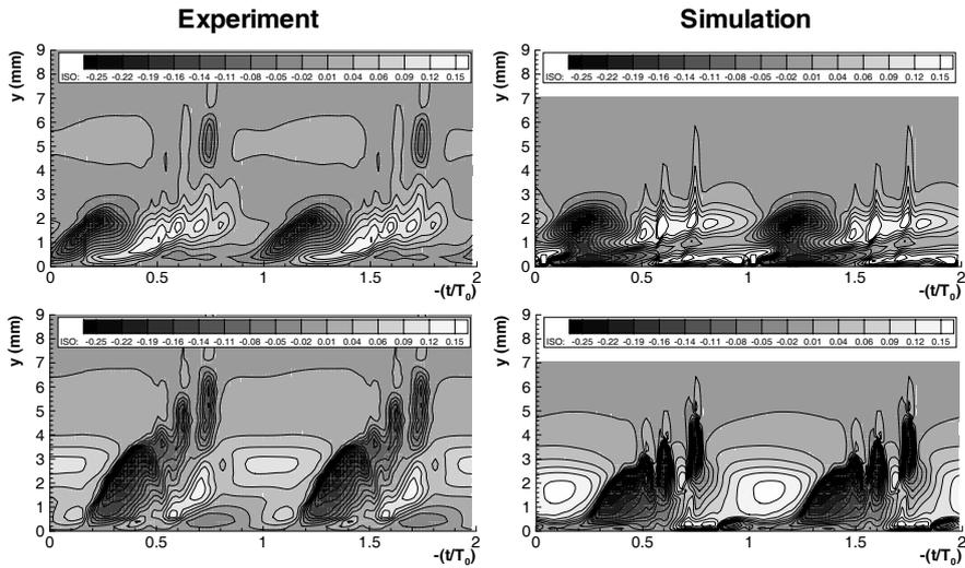
**Fig. 3.** Comparison of the  $u'$  component of experiment (left column) and simulation (right column) at 3-spike stage. Top row  $\Delta z \approx 2 \text{ mm}$  off-peak, bottom row at peak position  $z = 0 \text{ mm}$
