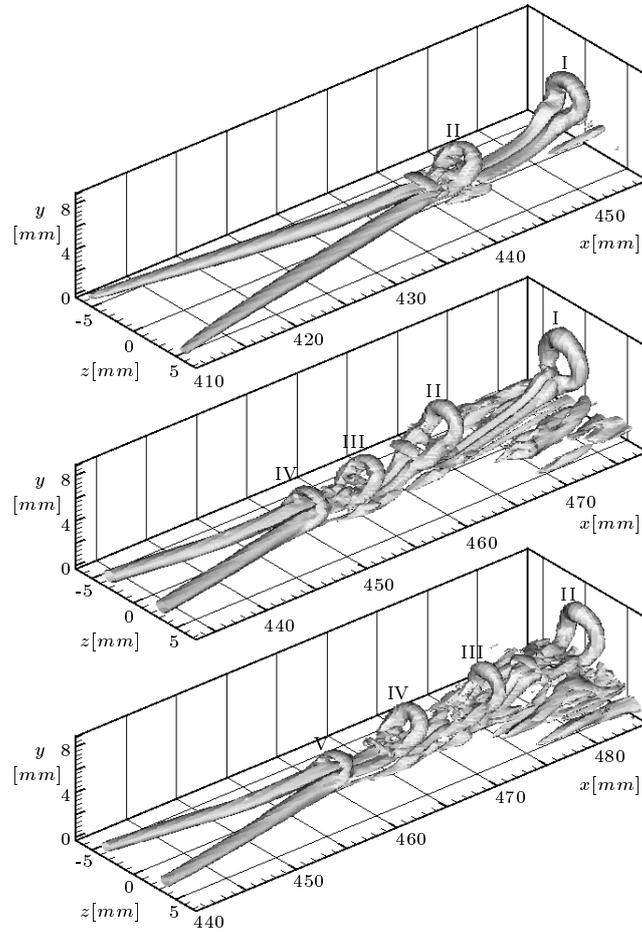
**Fig. 1.** Iso-surfaces  $\lambda_2 = -200$  for three time instants,  $t/T_0 = 0.335$ ,  $0.605$ , and  $0.845$ , from top to bottom, respectively
